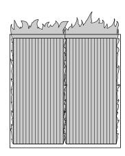
Figure 20 - Incorrect Burner Flame Pattern (Model VP11 Shown)
